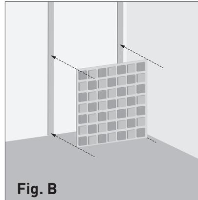
2) Fit the panel to a frame of wooden strips using countersunk bolts .
