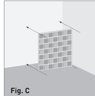
3) Fix the panel to the wall by drilling holes and using the right dowels and screws.
