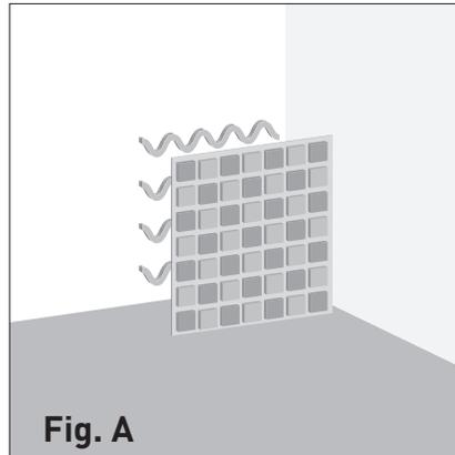
1) Attach the panel to the wall using a fitting mounting adhesive.
